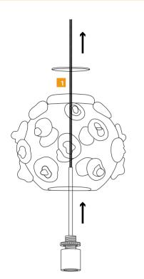
Feed coaxial cable as shown through applicable glass.
