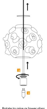
2 Rotate to raise or lower glass leveling nut. Raise or lower and fine adjust nut level so top of socket holder (threaded part) is level with top of glass.
